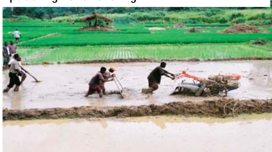
Figure 5: A power tiller in use in Nigeria for “puddling” and leveling
